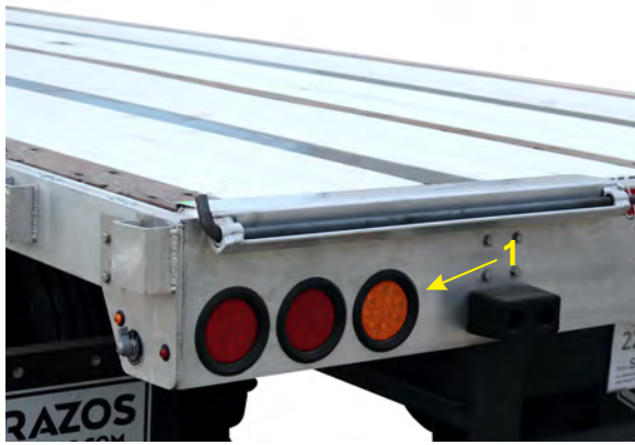
Figure 3-20 – Step Deck Safety Hazard Lights
