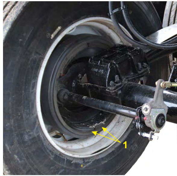
Figure 4-17 – Brake Shoe Lining Inspection
