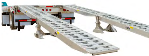
Figure 3-30 – Double Ramp System
