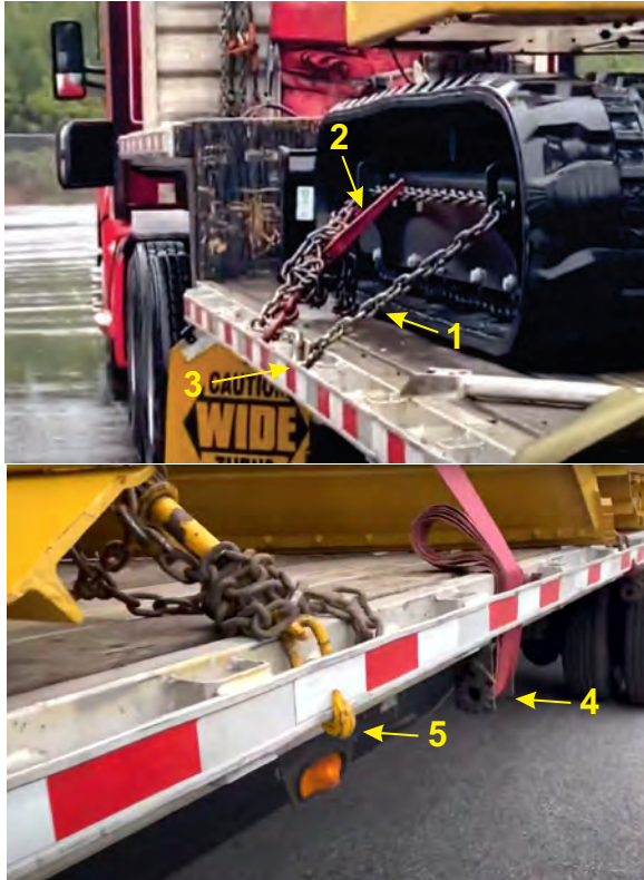
Figure 3-17– Loaded Secured with Chains, Binders and Straps
