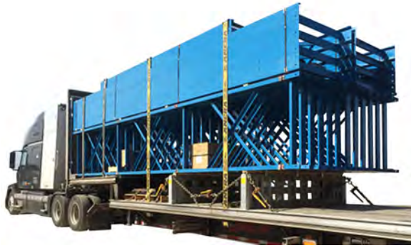
Figure 3-36 – Level Load Using Step Deck
