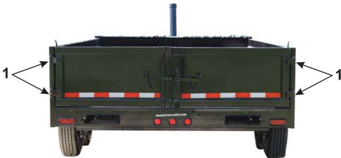
Figure 4-10 – Tailgate Grease Zerks
