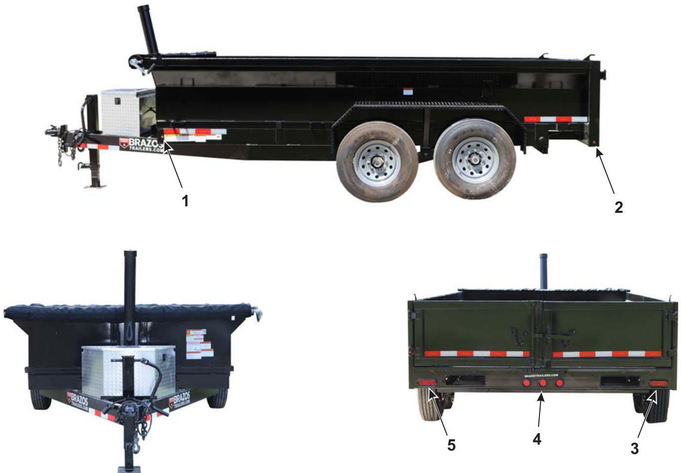
Figure 3-31 – Bumper Hitch Dump Trailer Marker, Stop and Turn Signal Lights
