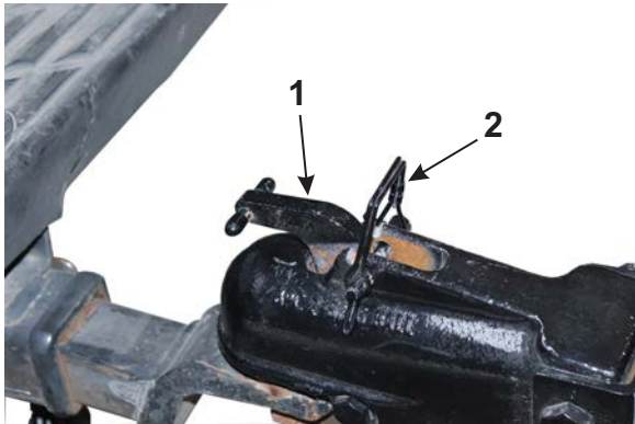
Figure 3-7 – Locked Coupler and Quick Clip
