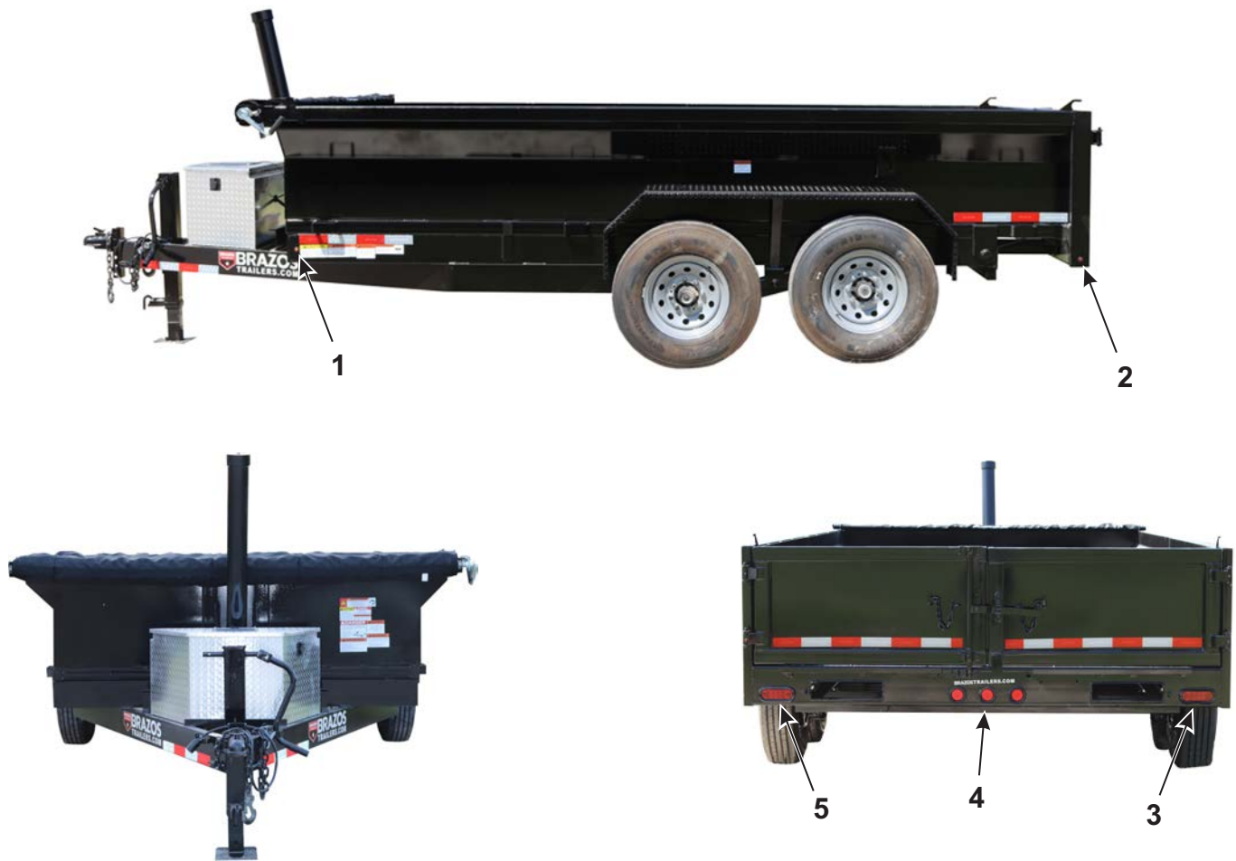
Figure 4-3 – Bumper Hitch dump Trailer Marker, Stop and Turn Signal Lights
