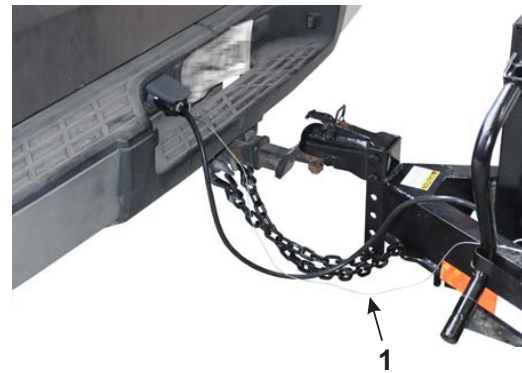
Figure 3-10 – Breakaway Brake Lanyard
