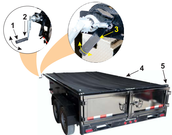
Figure 3-13 – Tarp in Travel Position
