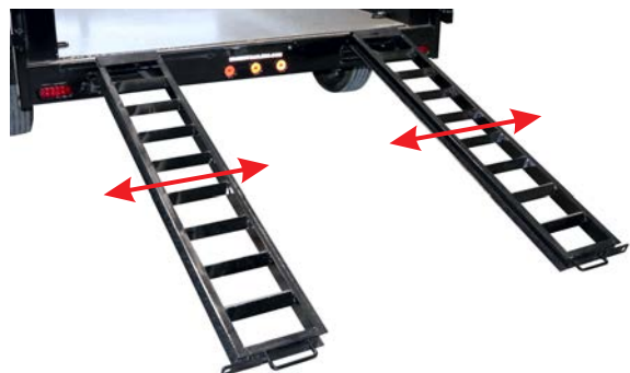
Figure 3-28 – Adjust Ramp Width
