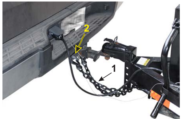
Figure 3-8 – Attach Trailer Safety Chains
