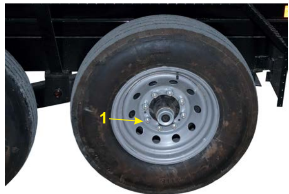
Figure 4-16 – Check Lug Nuts
