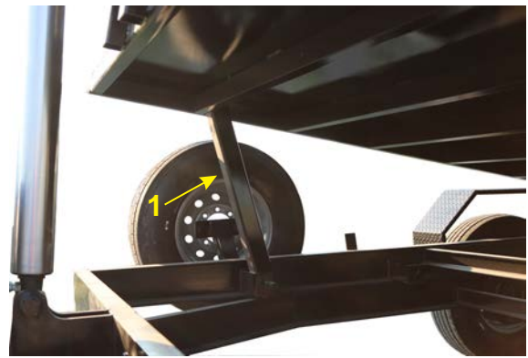
Figure 4-15 – Dump Body Service Support
