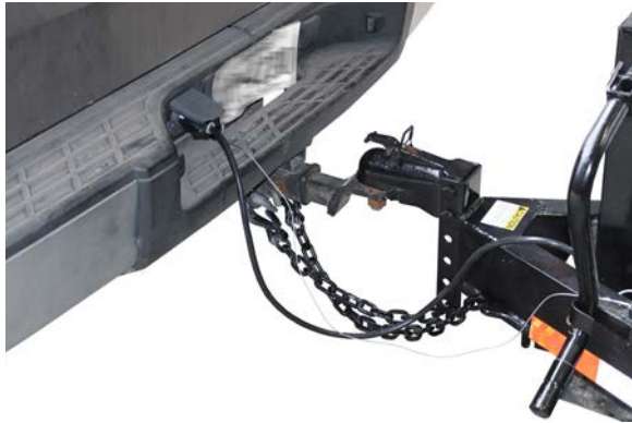
Figure 3-24 – Trailer Properly Attached to Tow Vehicle
