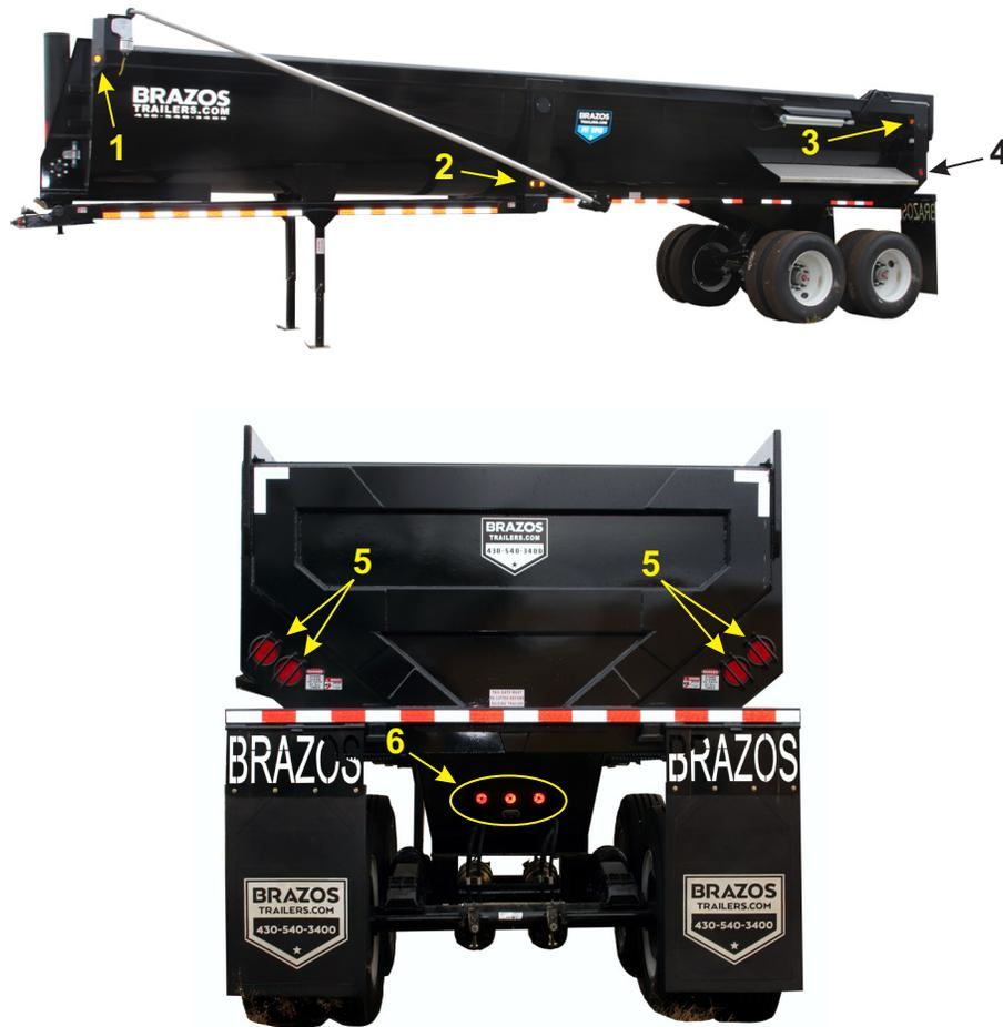
Figure 4-5 – Semitrailer Marker, Stop and Turn Signal Lights
