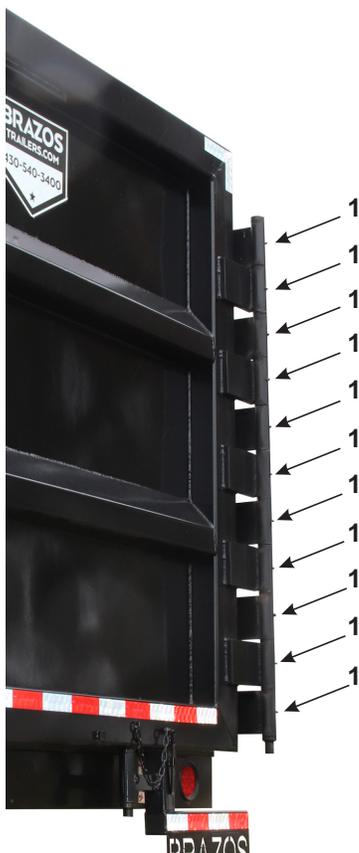
**Figure 4-10– Manual Tailgate Grease Zerks**
