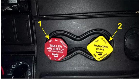
**Figure 4-7 – Tractor Air Supply Controls**
