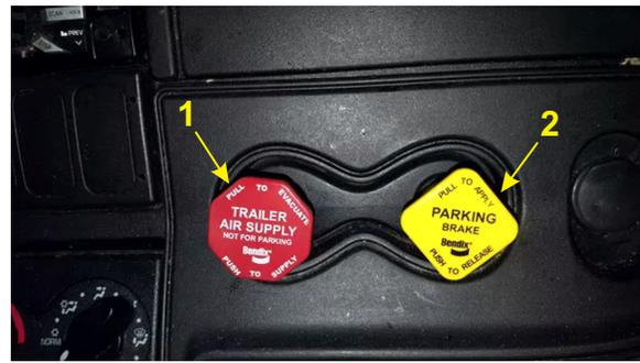
**Figure 3-12– Tractor Air Supply Controls**
