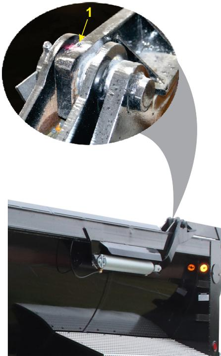
**Figure 4-9 – High Lift Tailgate Grease Zerks**
