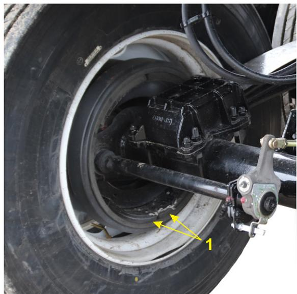
**Figure 4-12 – Brake Lining Inspection**
